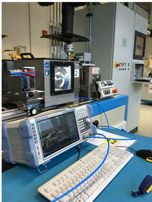
Figure 7: Test bench setup for impedance spectroscopy during dynamic operation
