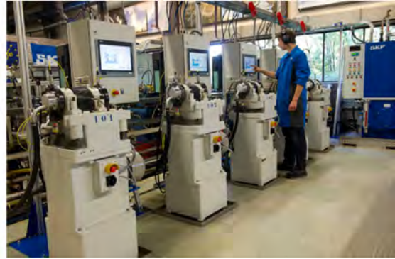
Figure 10: Left: a drawing of an example bearing life test rig; Right: a picture showing a battery of bearing test rigs.
