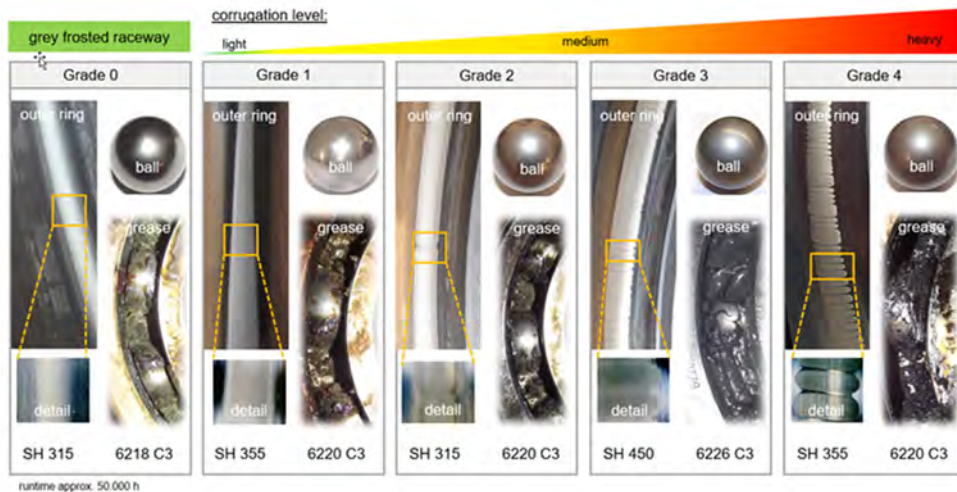
Figure 1: Different degrees of bearing damages [2, 3, 4]
