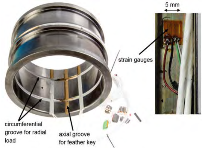
Figure 6: One inner ring of the planetary bearing with circumferential grooves for the integration of strain gauges.
