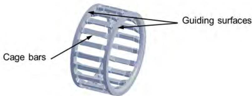
Figure 2: Model of the cage consisting of two guiding surfaces and a certain amount of cage bars
