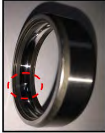
Figure 5: Artificially outer race defective ORS6205 ball bearing.
